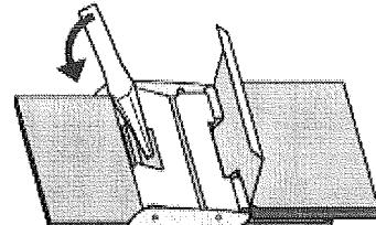
2. Place a small tool like a screwdriver in the slot to lift the bar according to the image.
