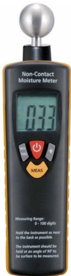
The NON-Contact Moisture Meter is an electronic dampness indicator with a measuring process working on the principle of high frequency measurement. The instrument is used for non-destructively tracing dampness in building materials of all kinds as well as for detecting damp distribution in walls, ceilings and floors. It is particularly suitable for pre-testing the readiness of building materials for covering prior to CM measurement.
