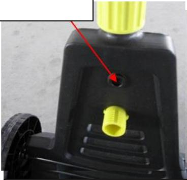
Step 4: Insert the nut and screw the screw behind through the hole in the tube.
