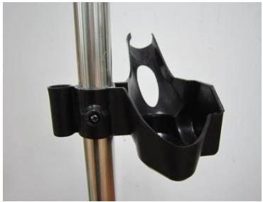
Step 6: Adjust the gun support to the desired height and use the small screw to secure it.
