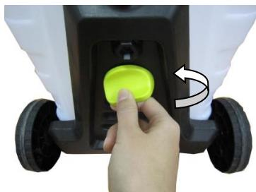
Step 2: Separate the tank and the base by loosen the yellow button
