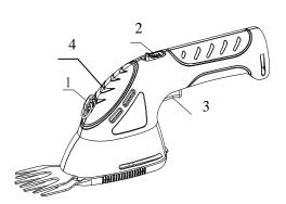
2. Push lock-off button (2) forward and press switch (3).
