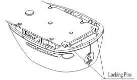
3. Lightly tilt the blades and insert into the grass and hedge shear. Make sure the blades fit under both locking pins. Press the blades down.
