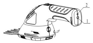
(1). Connect the power cord of the charger with a wall socket and the charging socket (1) of the grass and hedge shear.The charging indicator lamp (2) lights red.
