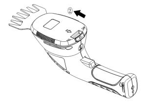
4. Place the blade cover on the grass and hedge shear and slide the cover in direction to the blades until it locks noticeable.
