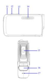
(1) Shutter key (2)Shaft (3) Hang rope buckle (4) Display screen (5) AV port (6) TF card slot (7) USB port (8) Power key (9) Mode switch key (10) Menu key (11) Charger light (12)W key (13) T key(14) Loudspeaker (15) Lens (16) LED fill light (17) Microphone
