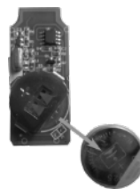
Image 27: Remove battery holder
