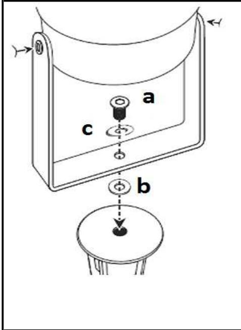
1. First unscrew the hexagonal socket head screw, which is screwed above the stake, with the Hexagonal key. Remove this screw and the washers.
