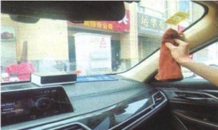
4. Install the sucker on the side of the main driving position
