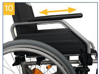
To swivel the armrest backwards, engage the release lever at the front of the arm rest and hold it down while simultaneously pulling the armrest up until the armrest is free. Now it can be swiveled backwards (**photo 11+12**).
